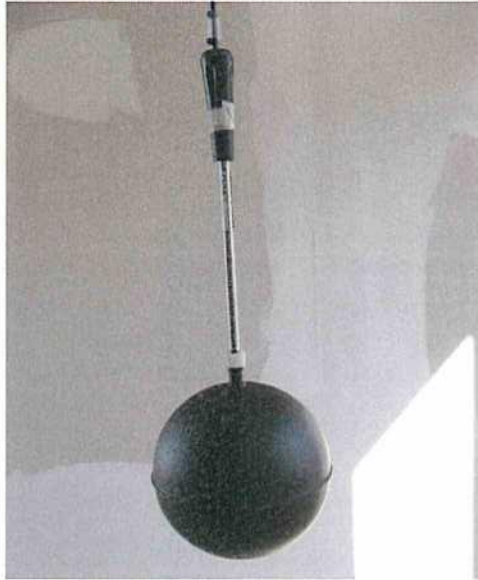
Figure 5. Globe thermometer for the measurement of the radiant temperature
