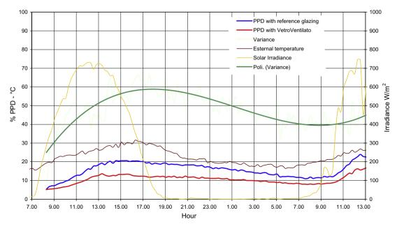
Fig. 6. PPD comparison in a typical summer day – slat angle of the shading component  $\alpha=60^{\circ}$  and  $\Delta T=2$  °C.
