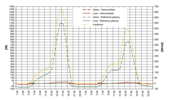
Fig. 14. Hourly solar gains vs loss for the west front of the case study concerning the office building located in Milan.
