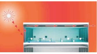
Vetroventilato® evacuates the heat of the windows thus lowering the internal temperature. All perimeter zones can be used comfortably.
